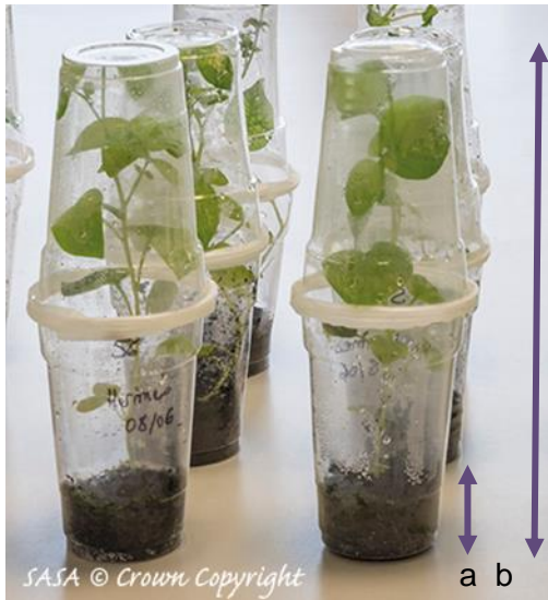
Figure 3. Microcosm set up used for assessing the growth of microplants in different growing media. a=35 mm depth of growing medium; b=360 mm microcosm height.
